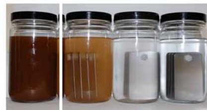
Increasing Inhibitor Concentration from Left to Right.
