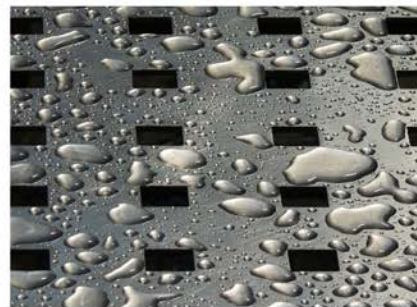
Increasing Inhibitor Concentration from Left to Right.
